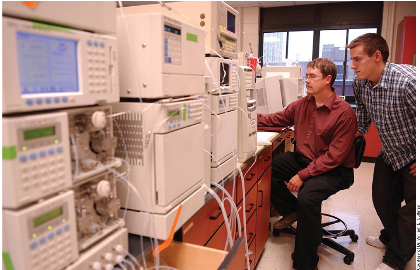
Dr. David A. Baker, assistant professor of biomedical sciences, and senior Jason Komp of Hartford, Wis., examine brain neurotransmitter levels using a high-performance liquid chromatography apparatus. The researchers are tracking changes in brain chemistry that accompany the addiction process.
